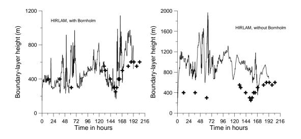
Simulation with the simple, applied model of the evolution of the boundary-layer height over Christiansø during the extensive observation period. In the left panel the effect of Bornholm is taken into account, in the right panel Bornholm is replaced by water. Crosses show measurements.
