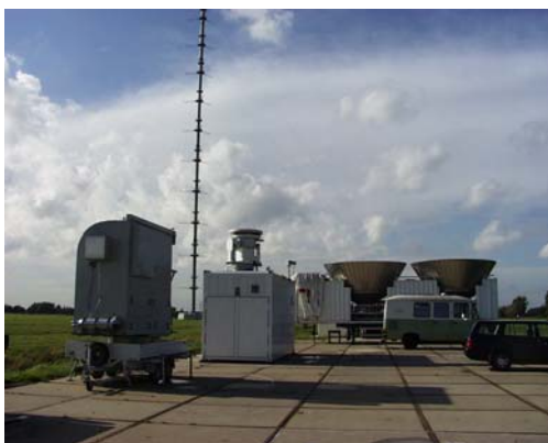
Figure 13.3: Set-up of the remote sensing site in Cabauw showing the microwave radiometer MICCY and three cloud radars. The 200 m mast is visible in the background.
