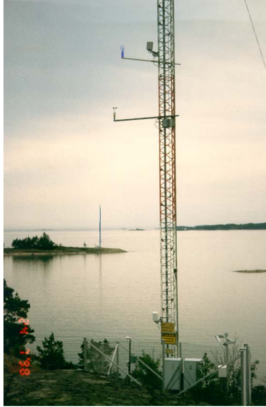
Figure 6.2: Kopparnäs. In the front the 50 m tower, and in the back the 33 m tower. The temperature of the sea water is measured at 0.5 m depth.
