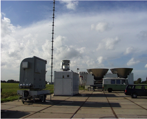
Figure 4: Set-up of the remote sensing site in Cabauw showing the microwave radiometer MICCY (far left) and three cloud radars. The 200 m tower is visible in the background.
