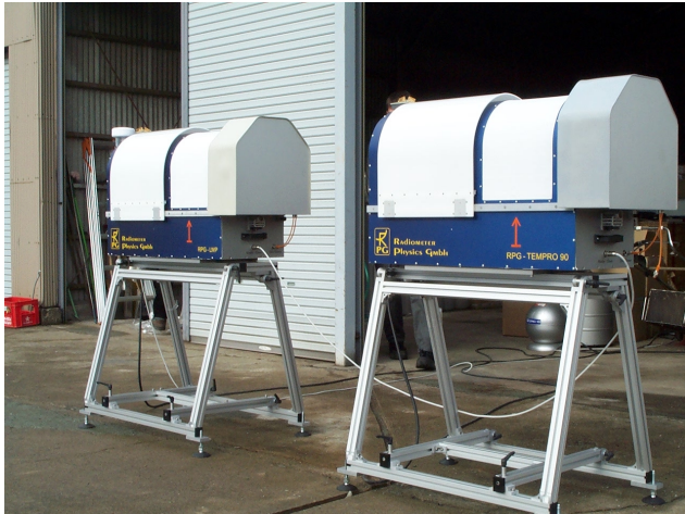
Figure 11: RPG-LWP and RPG-TEMPRO90 in a Master/Slave configuration. Both instruments are operated by the same host computer and configure themselves automatically as Master or Slave instruments due to their interface connections.
