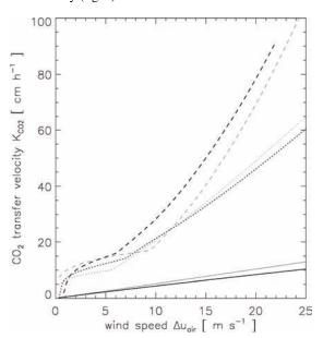
**Figure 2.** Wind-dependent CO2 transfer velocity for different wave ages (0: solid; 5: dashed; 25: dotted) for the analytical solution (thick) and the limiting cases (thin).
