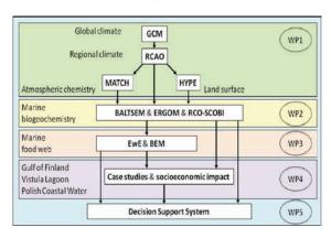
**Figure 1.** Model hierarchy in the ECOSUPPORT project and work package (WP) structure (see <a href="http://www.baltex-research.eu/ecosupport">http://www.baltex-research.eu/ecosupport</a>). The schematic is highly simplified neglecting complex interactions (e.g. fish predation pressure on zooplankton, changing society/policy will affect climate and nutrient load scenarios).
