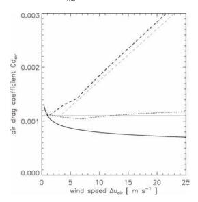
**Figure 1.** Wind-dependent drag coefficient for different wave ages (0: solid; 5: dashed; 25: dotted) for the analytical solution (thick) and the fit (thin).
