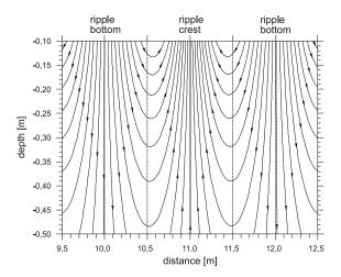
Figure 2. Stream function under ripple crests and bottom
