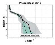
**Figure 3.** Average (1970-2005) phosphate concentration at BY15. The black solid line and the grey shaded area indicate the mean value and  $\pm 1$  standard deviation of BED data. The black dashed line and the blue shaded area indicate the mean and spread of the models ERGOM, RCO-SCOBI and BALTSEM.
