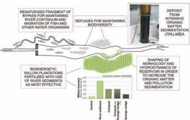
**Figure 2.** Example of "environment friendly" dam solutions.
