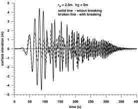
**Figure 2.** Surface oscillation close to waterline at water depth h = 5m
