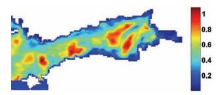
**Figure 2.** The North-South component of the average net transport in the Gulf of Finland over August–October 1988 based on the analysis of quasi-two-dimensional trajectories of water particles in the surface layer calculated with the use of the TRACMASS trajectory tracing code (Döös 1995) and precomputed current fields from the Rossby Centre (Swedish Hydrological and Meteorological Institute) circulation model (Meier 2001).
