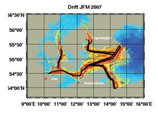
**Figure 4** Endpoints of drift tracks after 5 (red dots) and 10 days (yellow dots) for winter (DJF) 2007. Drifters have been released in a distance of 2 km along the ship routes (black lines)
