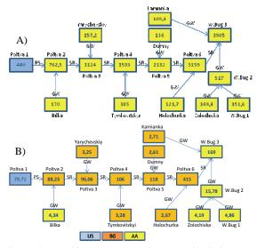
Figure 4. Resulting TN (A) and TP (B) loads in W.Bug basin. Numbers in the boxes are resulting loads at the outlet of the sub-basin; color of boxes correspond to the main sources: US – urban system, BG – background, AA – agricultural areas; the pathways are designated as following PS – point sources, GW – groundwater, SR – surface flow.
