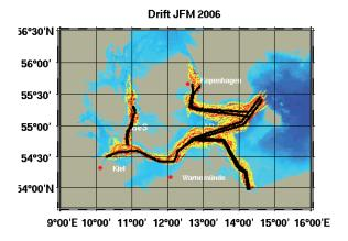
**Figure 3** Endpoints of drift tracks after 5 (red dots) and 10 days (yellow dots) for winter (DJF) 2006. Drifters have been released in a distance of 2 km along the ship routes (black lines)
