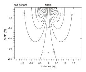
Figure 1. Stream lines pattern below a single ripple
