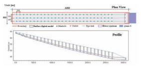
**Figure 3:** Setup of conceptual model. It has been designed to be a regular Danish catchment with flat and small subareas. The sewer is designed for return period T=2 years storm event.
