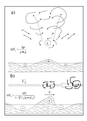
**Figure 1**. Diagram of sea surface deformation casued by a low pressure system
