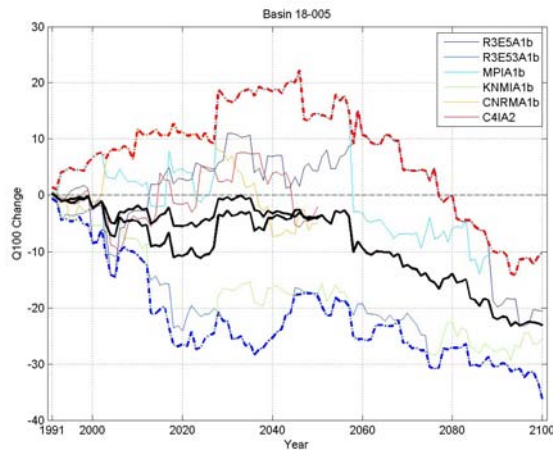
Figure 3. Example of the development of 100-year floods according to a number of climate scenarios for River Byskeälven in northern Sweden. The scale is percent change in relation to the reference period 1961-1990.
