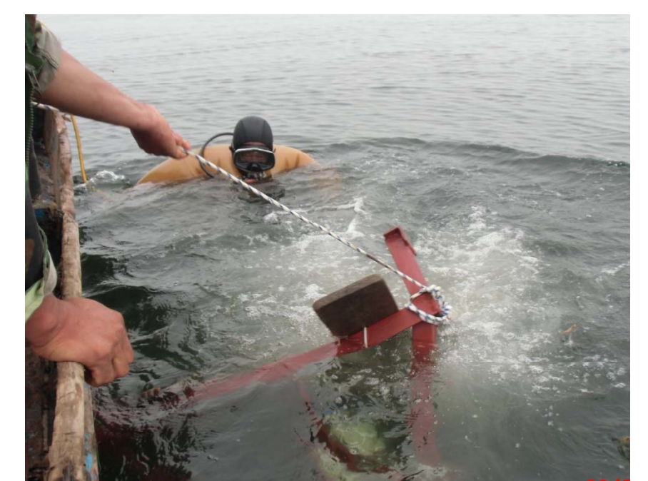
Fig.5 Left: The ADCP before deployment, Right: ADCP put in the water with diver help
