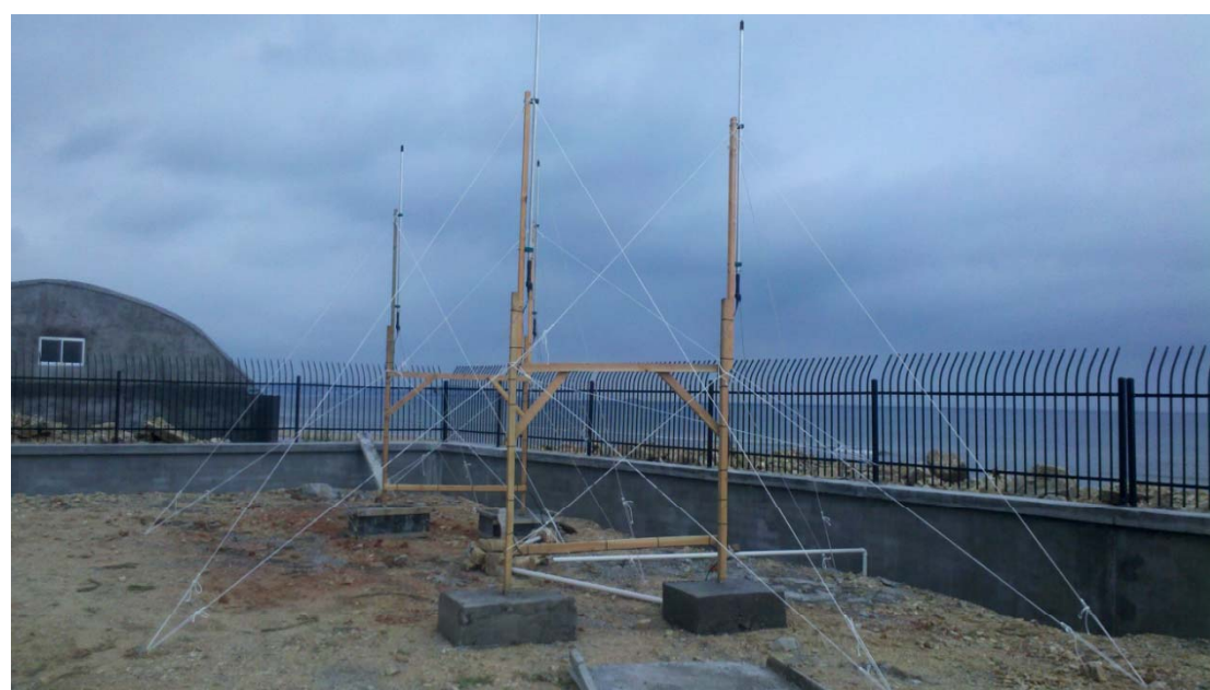
Fig.1 Left: The installed transmit antenna in site 1, Right: the plotted range of HF radar installed in Yantai coast
