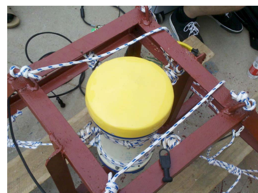
Fig.5 Left: The ADCP before deployment, Right: ADCP put in the water with diver help
