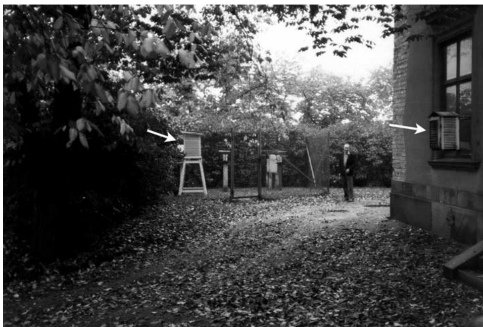
Figure 3. The window screen (at the right arrow) where temperature was measured from 1878 to 1960 and the SMHI screen (at the left arrow) which has been used since 1961. The photograph was taken in October 1984. (Photo: SMHI).
