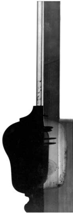
Figure 10. X-ray image of the lower part of Ekström's barometer. (Image: Stiftelsen Observatoriekullen).
