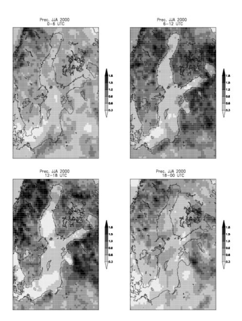
Figure 1. The average amount of precipitation in June, July and August, 2000, given by the BALTEX/BRIDGE reassimilation system (forecast hours 6-12) as a function of the time of the day. The unit is mm in six hours.
