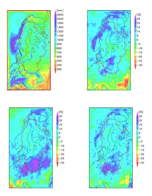
Ten year mean precipitation in mm/year for the control run (1990 to 1999, upper panel left) and changes in percent for the following decades:
