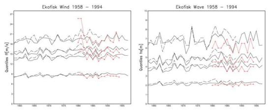
Figure 3: Annual 50, 90, 95 and 99% iles of wind speed and significant wave height at Ekofisk. Red: observations. Dashed: WASA project results (based on high res. DNMI analyses). Solid: Results obtained from regional climate model (Weisse and Feser, pers. comm.)
