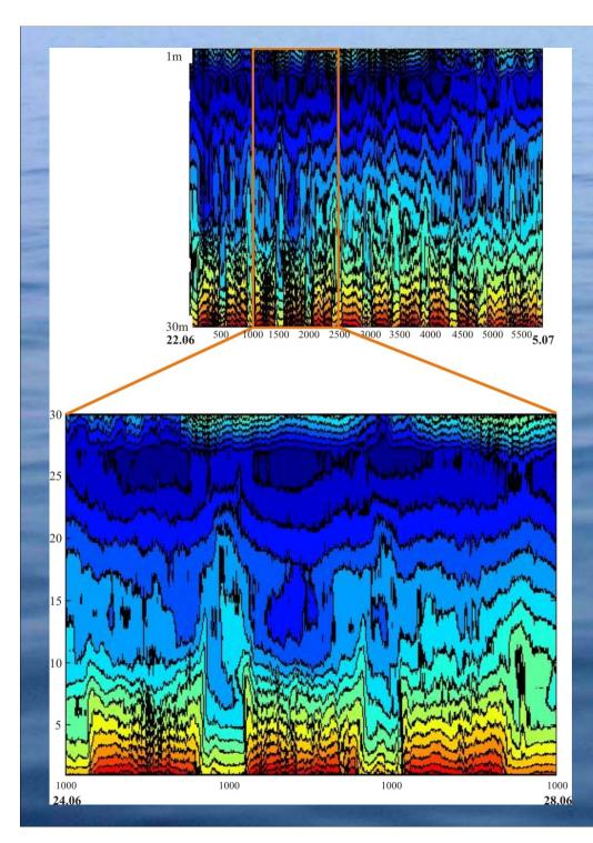
Near the offshore platform the autonomous acoustic bottom station (ADCP) continued permanent measurements of currents and suspended matter concentrations
