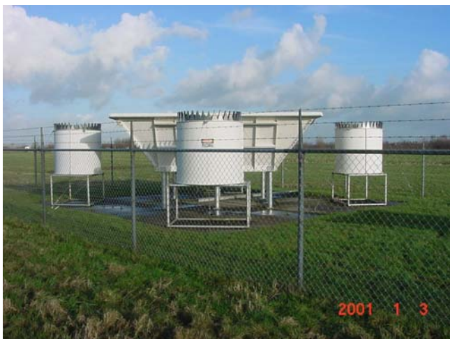
Figure 3: The 1290 Mhz wind profiler/RASS system which give wind and temperature profiles in the atmospheric boundary layer.
