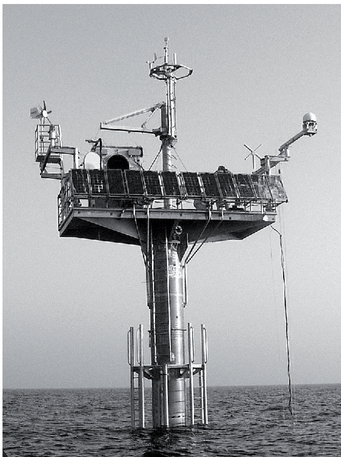
Figure 5. MARNET station Arkona Sea. At the right hand side of the platform, the GPS antenna and the radar gauge can be seen.
