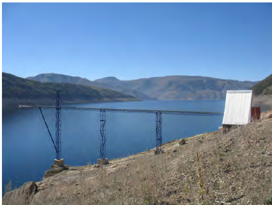
Figure 5. GNSS-R instrument over Laja Lake, Los Angeles, Chile, for monitoring lake level.
