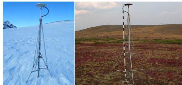
Figure 7. The GNSS station NWOT in Boulder, CO, USA used to measure snow depth by means of reflections of GNSS signals (© K. Larson, Univ. of Colorado).
